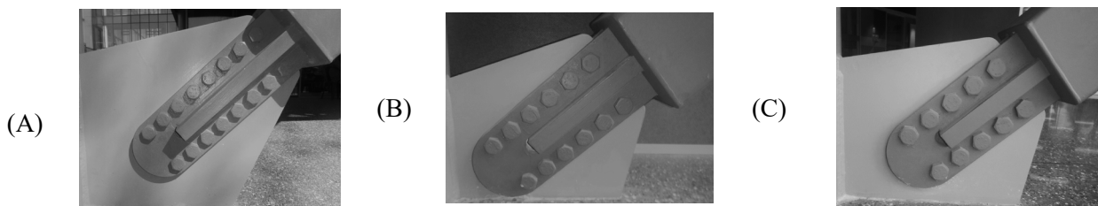
Figure 4. Various lengths of bolted connection arrays used in BRBF design (A) 16 bolt array. (B) 12 bolt array and (C) 10 bolt array
