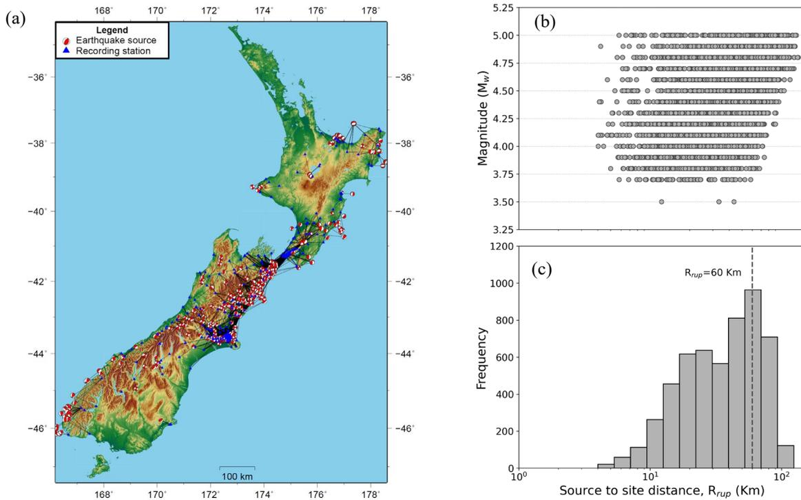
Figure 1: Descriptions of the simulated and observed ground motion sets considered in this study a) 496 small-magnitude events, 5349 strong motion stations, and schematic observed ground motion ray paths; b) distribution of magnitude versus source-to-site distance; and c) source-to-site distance histogram.
