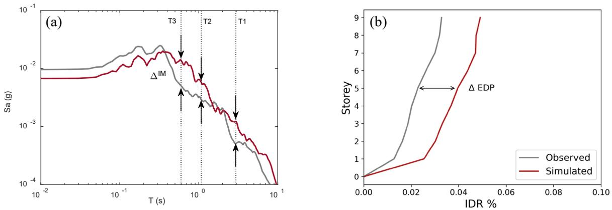
Figure 3: Comparison between the simulated and observed a) response spectra; b) structural response (IDR) along the height of 9-storey model.
