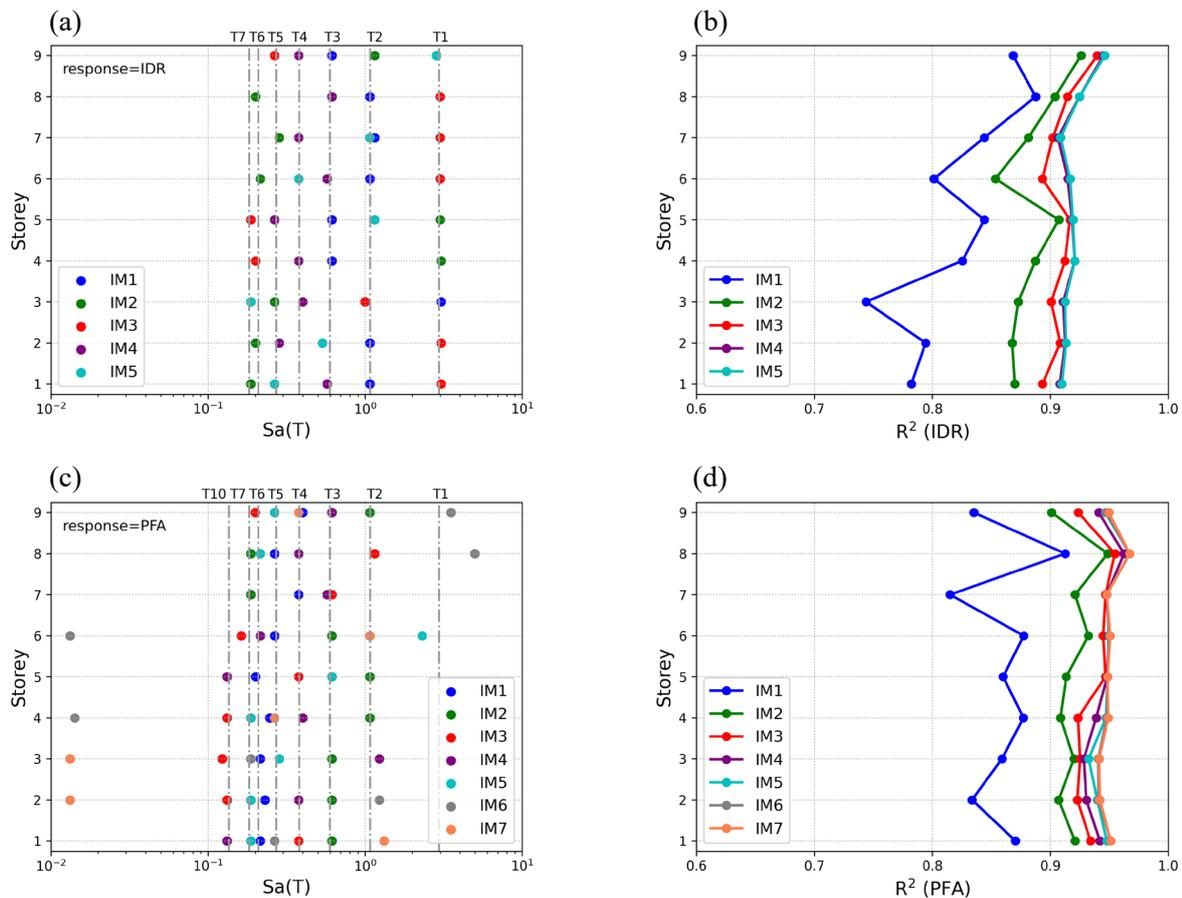
Figure 6: Variable selection and coefficient of determination ( $R^2$ ) for Building B a-b) IDR; c-d) PFA.
