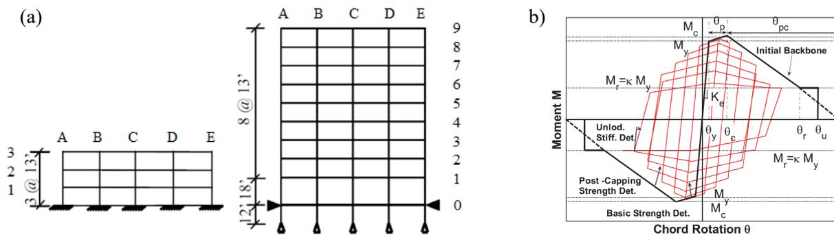
Figure 2: a) Schematics of SAC steel frames (FEMA 2000); b) Hysteretic behaviour of the plastic hinges (Lignos 2008).
