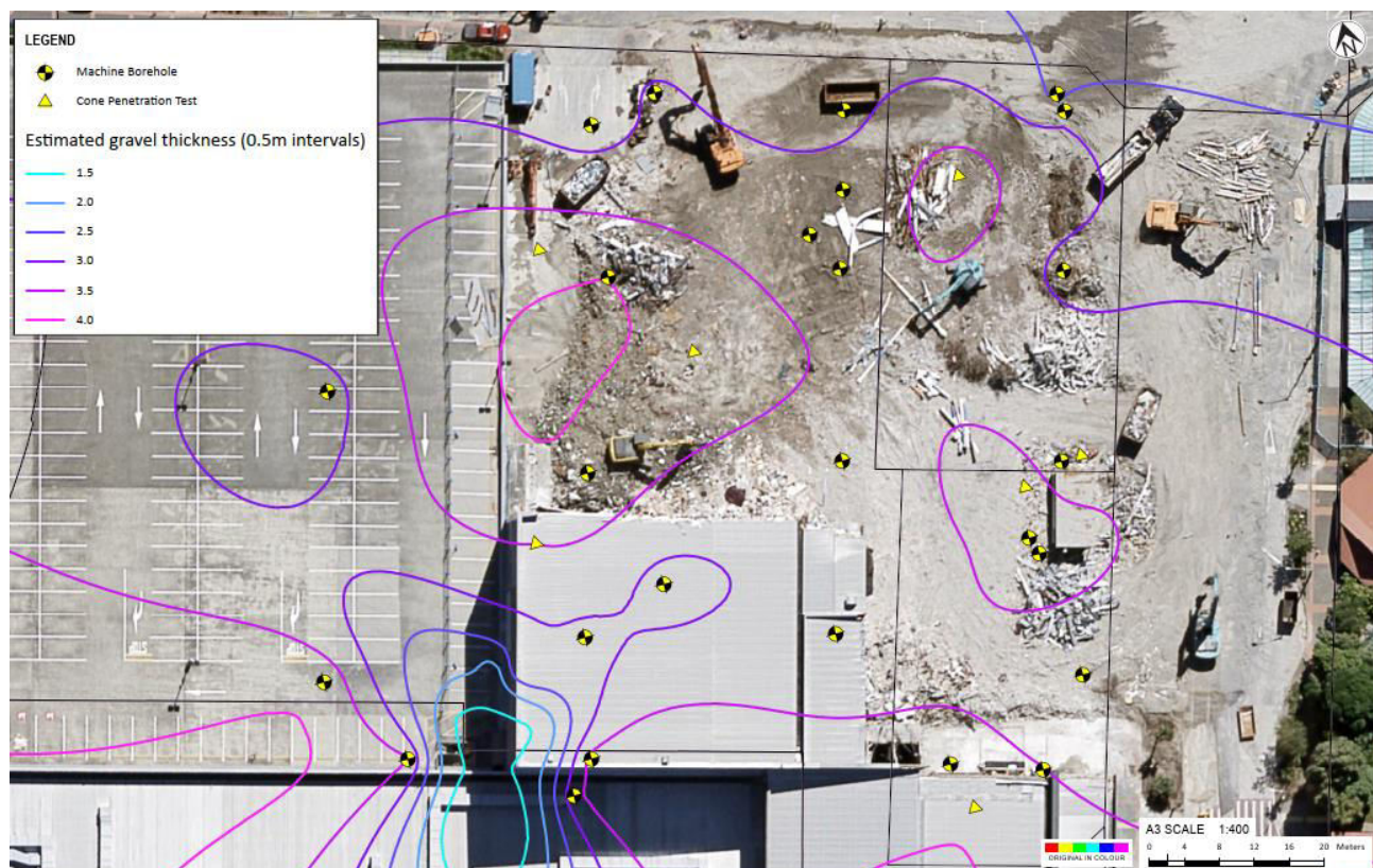
Figure 2 Contours of the thickness of the founding gravel layer at the site.
