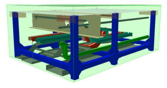
Figure 1- 3D view of modelled services and cradle frame
