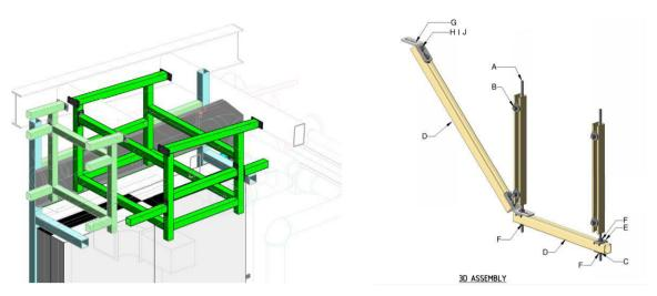
Figures 2 and 3- 3D of cradle for shared service and 3D of trapeze for individual restrained services
