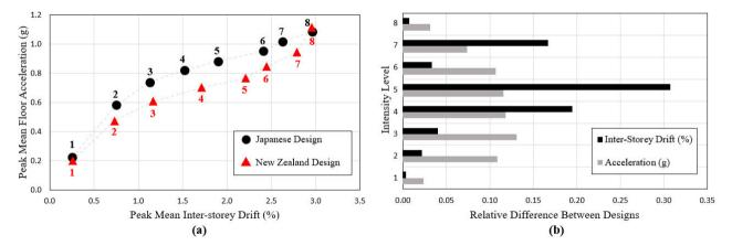
*Figure 6: IDA results; (a) Peak mean inter-storey drift vs acceleration at each intensity level and (b) Relative difference of peak mean inter-storey drift and acceleration between designs at each intensity level*
