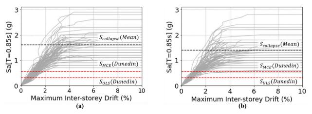
Figure 4: IDA curves; (a) Japanese design and (b) New Zealand design moment frames
