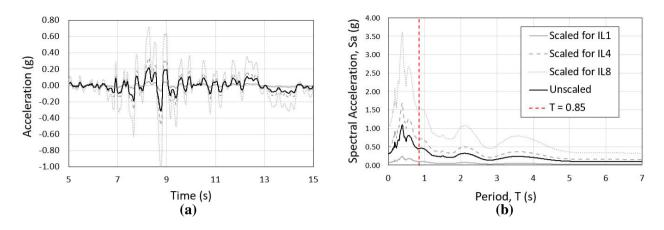
*Figure 3: Example of IDA scaling process; (a) unscaled and scaled ground motion input and (b) corresponding unscaled and scaled response spectrums*
