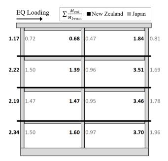
Figure 2: Column-to-beam moment strength ratios for New Zealand and Japanese moment frame designs
