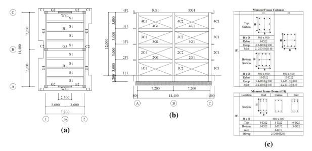
*Figure 1: Case study building; (a) plan view, (b) moment frame elevation, and (c) moment frame sections Note: all dimensions are in mm (modified from Nagae et al., 2015)*
