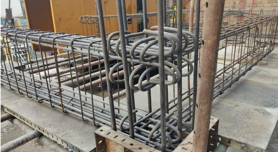
Figure 4: Longitudinal and transvers reinforcing of the specimen.
