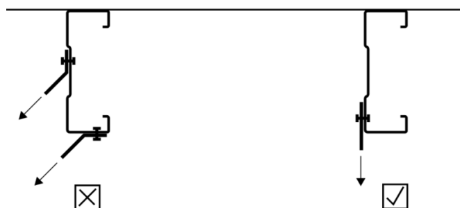
Figure 5. Connecting Seismic Restraint braces to light gauge purlins
