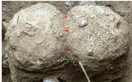
Figure 8: PPT measurement points (marked in red) between bulbs Up01 and Up02. Twelve months after their removal from the pit, the bulbs and the connection between them remain solid and stiff
