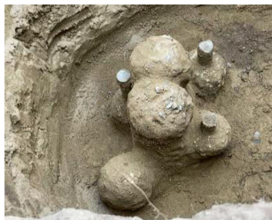
Figure 3: SCRR miniature consisting of six bulbs, with four bulbs in the base layer and two bulbs installed on top as the top layer. The bulbs have a diameter of 9 to 12 cm.
