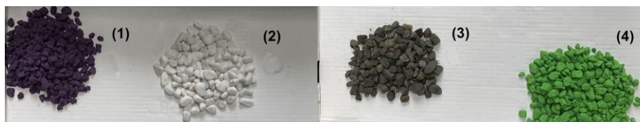
Figure 9: Photograph of the four batches of gravel (with each batch having a volume of approximately 1E^{-6} m^3 ) coloured purple (1), white (2), black (3), and green (4) used to produce one SCRR bulb. The batches were placed in the bottom of the hole in order and compacted.
