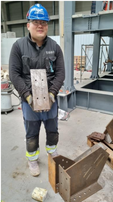
Figure 11. Zhenduo Yan Brace Shim Wear from Test 2c
