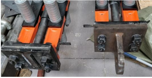
(a) Photo (see left cleat fracture)
