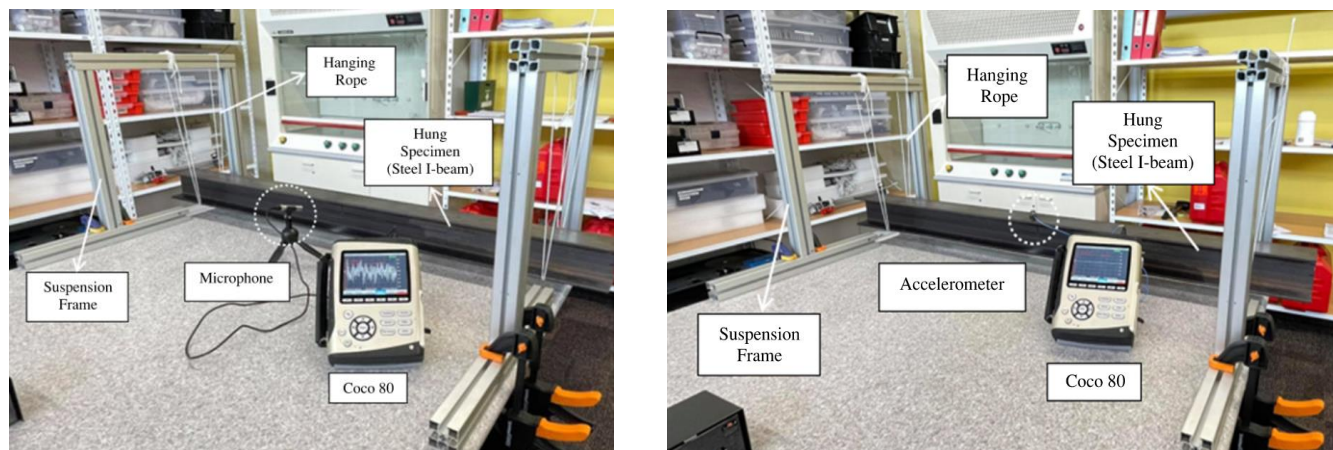
Figure 1 Microphone test setup (left); Accelerometer test setup (right).
