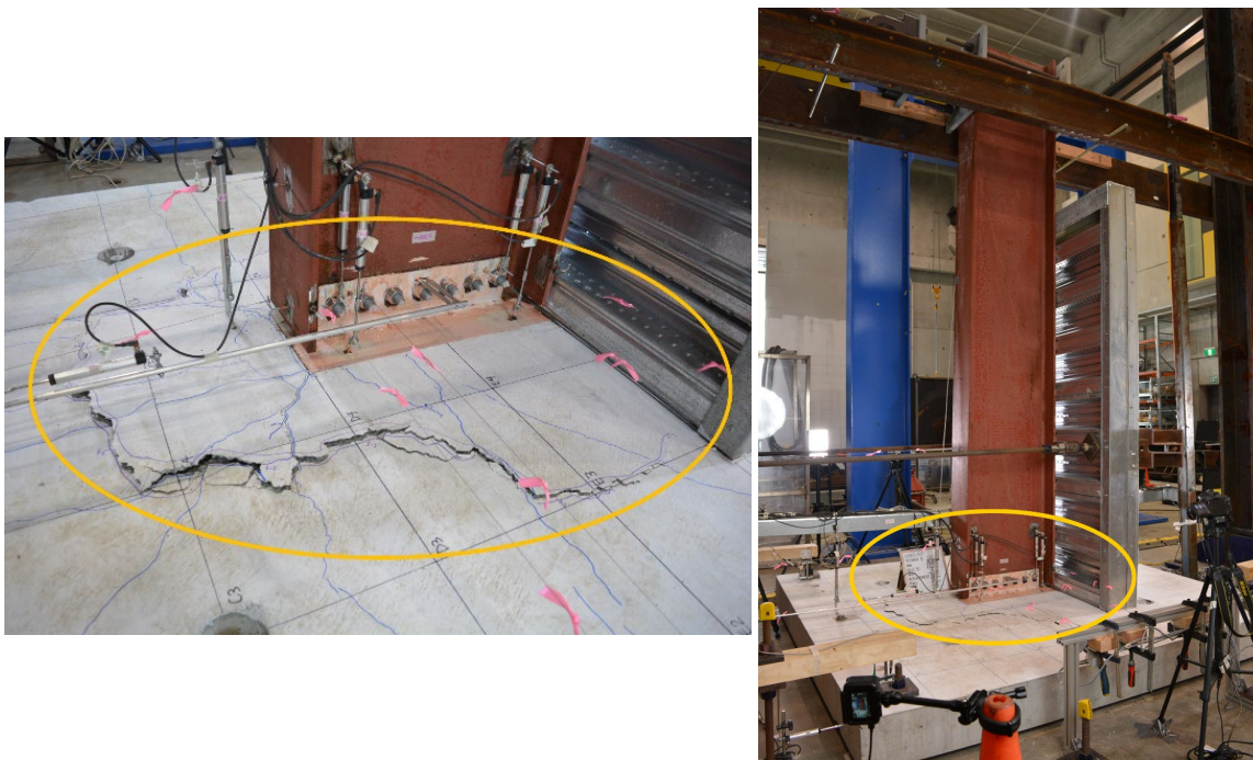
Figure 3: Concrete breakout failure in one of the test specimens
