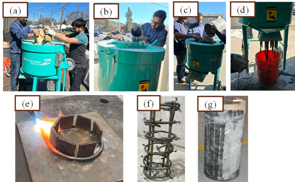
Figure 1. Preparation of UHPC (a) Addition of premix (b) Addition of superplasticizer and water (c) Addition of steel fibers (d) Discharging of UHPC mix (e,f) Preparation of TiAB ties (g) Confined specimen ready for test
