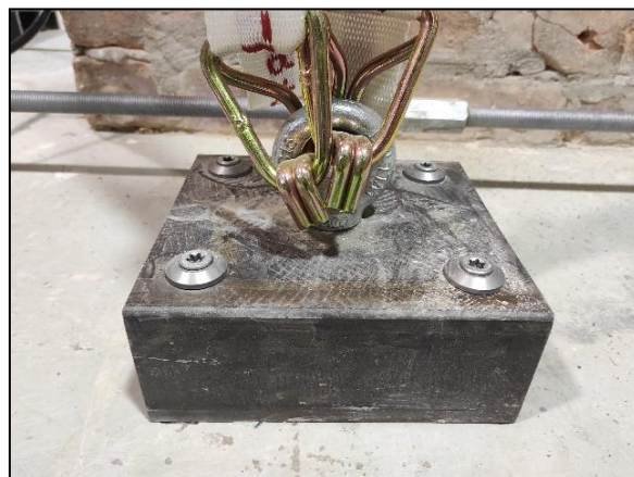
(b) Vertical loading anchor points to the floor
