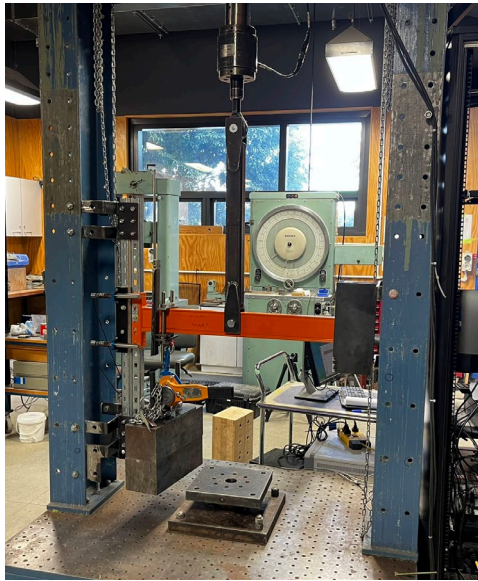
Figure 3: Test rig of beam end connector bending test with a specimen during testing
