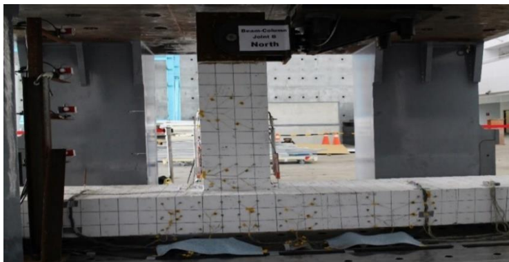
Figure 2: BCJ specimen test configuration utilizing MATS
