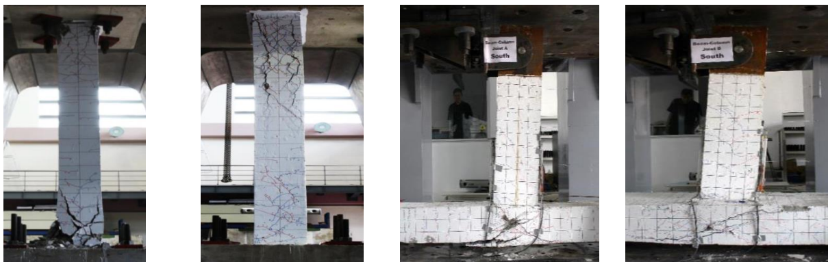
(a) C-A at 8% drift ratio (b) C-B at 4% drift ratio (c) BCJ-A at 5% drift ratio (d) BCJ-B at 7% drift ratio Figure 3: The final crack pattern at of the column and BCJ specimens, corresponding to different drift ratio
