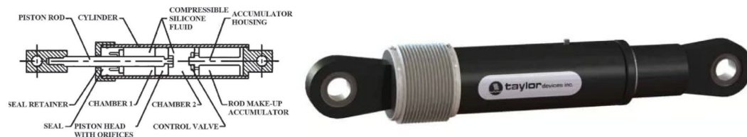
Figure 1: A typical cross section of a viscous damper (Taylor Devices inc.) and an assembled unit (Taylor Devices inc.)
