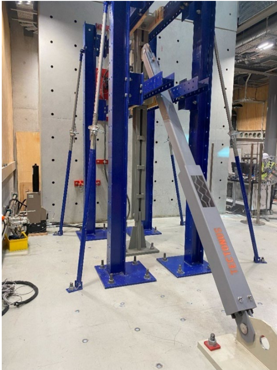
Fig. 10: Dynamic testing of DMAX brace with a capacity of 310kN
