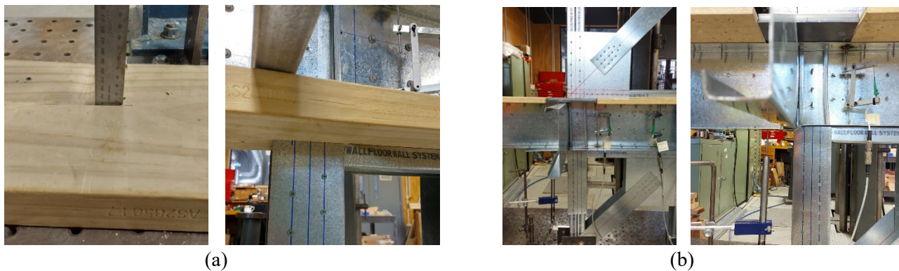
Figure 8: The crushing of the (a) horizontal timber in Test 8 and (b) boundary joists' bottom flange in Test 9
