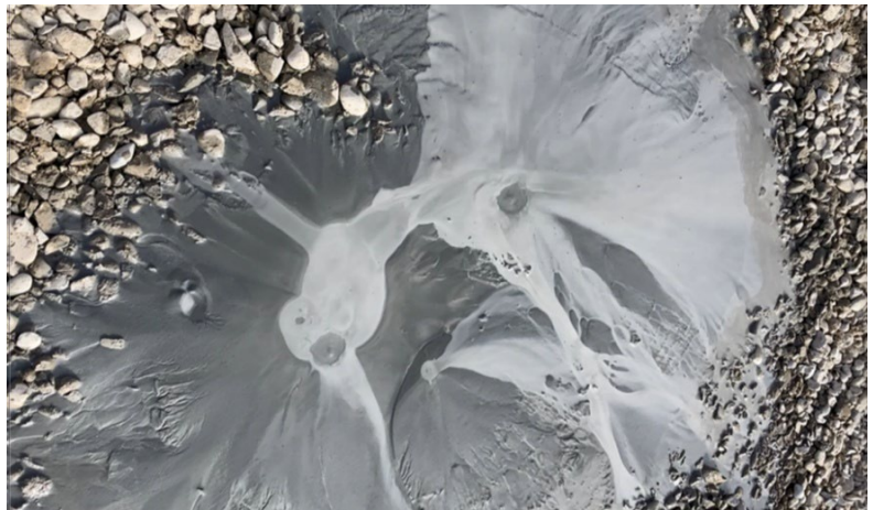
Figure 1: Paradox of drainage: Liquefaction occurrence at a RAPs installation site in Christchurch, 2023.
