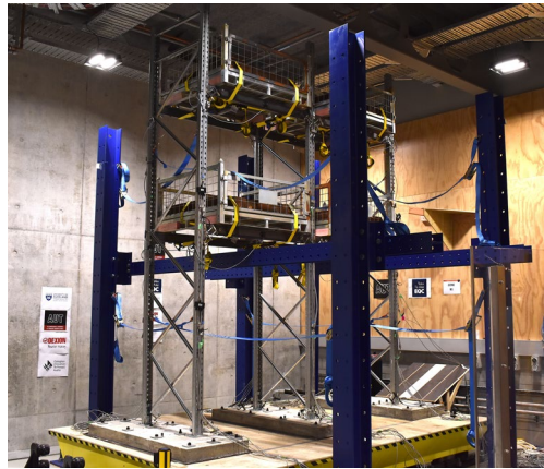
Figure 1: Full-scale two-bay, two-story pallet rack test specimen mounted on the AUT uniaxial shaking table with loaded pallets (1200 kg each), foundation blocks, and safety catch frame
