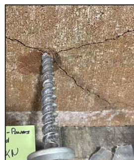
(b) Tension test - Splitting of specimen
