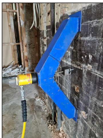
Figure 1: Example of tensile test setup
