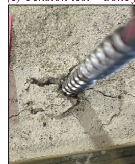
(f) Torque test - Threads bearing failure
