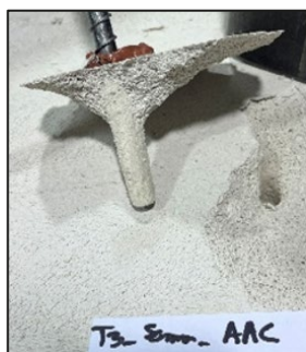
(a) Tension test - Cone and pull-out failure
