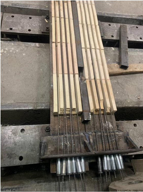
a) Ribs Following Prestressing of Wires
