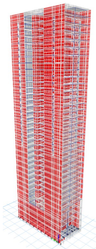
Figure 1. 34 storey building under design in Auckland (extracted from ETABS structural analysis programme)
