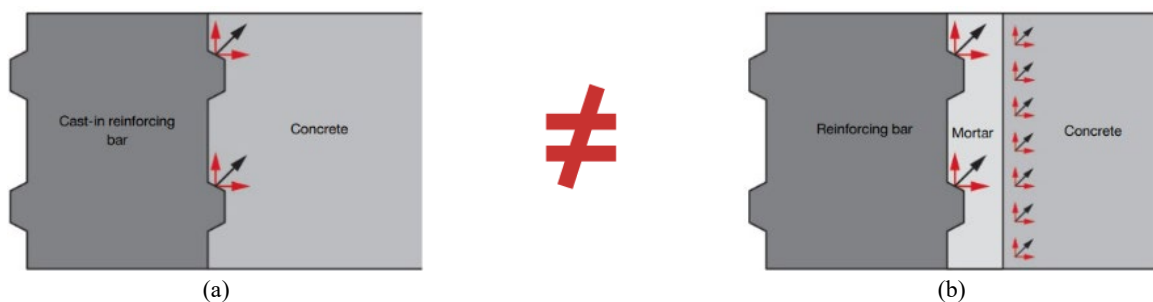
Figure 1: Working principles of Cast-in vs Post-installed reinforcing bars. Source: Hilti Corporation.
