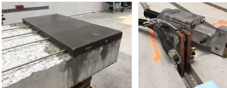
Figure 5: Cementitious end-anchorage (left) and shape memory activation with resistive heating (electric current), (Schranz et al., 2021)
