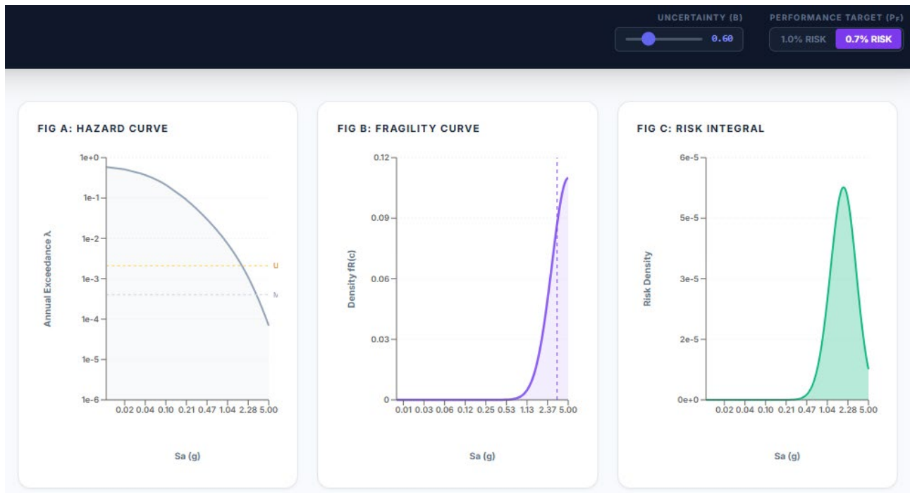
Figure 3: Hazard curve, fragility curve, and hazard-fragility integration for SA_{0.7\%} and \beta = 0.6
