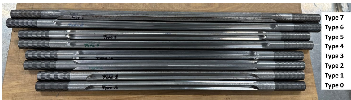
Figure 1: Steel fuse specimens (Types 0-7) prepared for experimental testing. During testing, these fuse cores are located within a thick-walled tube to prevent global buckling behavior.
